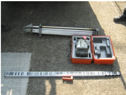
Settlement surveying system
